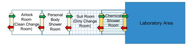
Figure 2: Simple schematic diagram of a suit containment facility. Entry into facility; Exit from facility. (Adapted from Biological Agents: The Principal, Design and Operation of Containment Level 4 Facilities. Advisory Committee on Dangerous Pathogens, United Kingdom.)
