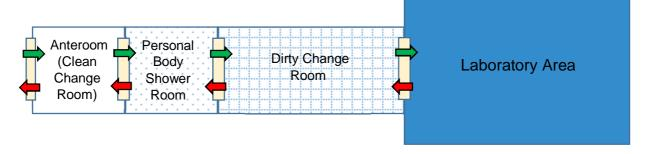
Figure 1: Simple schematic diagram of a cabinet containment facility. Entry into facility; Exit from facility. (Adapted from Biological Agents: The Principal, Design and Operation of Containment Level 4 Facilities. Advisory Committee on Dangerous Pathogens, United Kingdom.)
